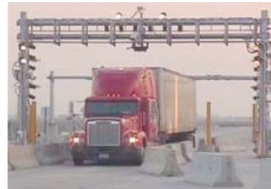
Equipment is electronically scanned while passing through portal
