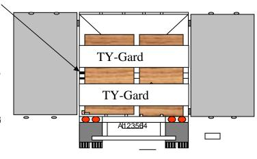
Ty-Gard can be used as a longitudinal restraint. Rule of thumb: 1 strip for every 8,800 lbs. of cargo. Must glue to side wall, minimum of 5 ft.
