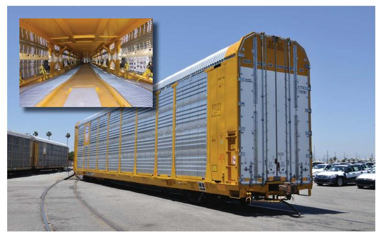
Developed by Union Pacific Railroad, the 90-foot long **AutoFlex™** rail car can be adjusted to accommodate bi-level or tri-level vehicle transport while using the same rack structure. The **AutoFlex** car will deliver numerous benefits to Union Pacific customers, including:
