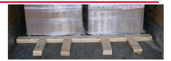
Floor blocking should be constructed with double 2x4 or 2x6 lumber with backup cleats, at least 18 inches long. Floor blocking needs to be as long as the pallet or unit it is supporting. Nails should be staggered and spaced approximately 4 to 5 inches apart. 16d nails (or larger) are required.
