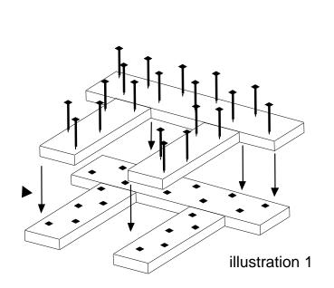
Floor blocking should be constructed with double 2x4 lumber with backup cleats, at least 18 inches long. Floor blocking needs to be as long as the pallet or unit it is supporting. Nails should be staggered and spaced approximately 4 to 5 inches apart. 16d nails (or larger) are required. Each 16d nail has a holding power of 950 lbs. Appropriate # of nails are required, based on lading weight.
