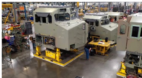
A main cab for a Union Pacific modernized locomotive.
