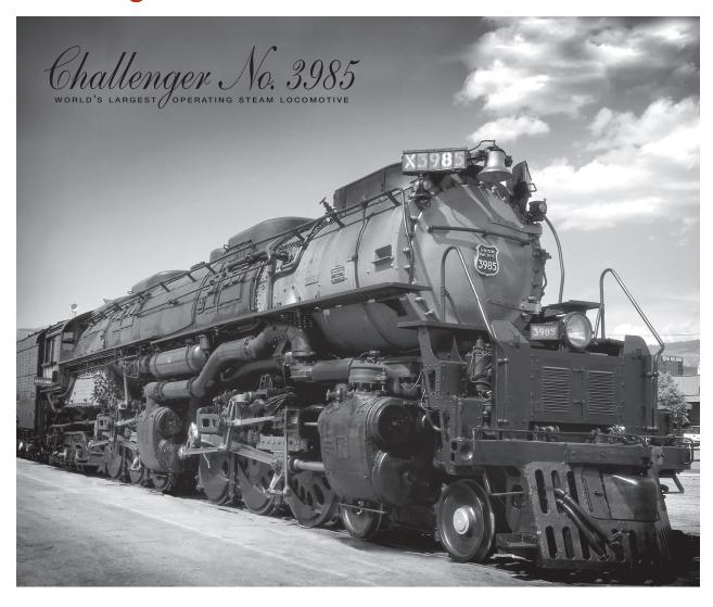
The Challenger No. 3985 was designed by Union Pacific and built in 1943 by the American Locomotive Company. It is one of 105 Challengers built for Union Pacific between 1936 and 1943 and is the only operating engine of its class in the world today – the largest and most powerful operating steam locomotive.
