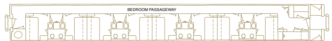
Configuration: Omaha is a Sleeper Car with eight bedrooms, each with a private restroom. The rooms share adjoining showers. (Sleeps eight guests)
