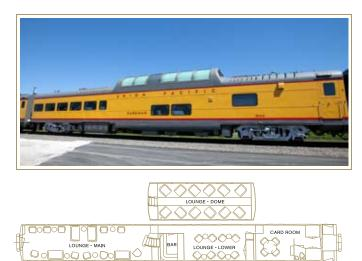
Configuration: Harriman is a Dome Lounge with a small room containing a card table and four chairs on the short end of the car, followed by a bar with seating for eight in the belly. The long end has seating for 18 and there is seating for 12 in the dome. Total car seating is 42.
