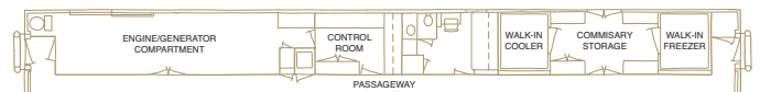
Configuration: UPP 207, UPP 208 and UPP 2066 are Power Cars with two Deutz diesels in one end and a control room. It has a crew room with private bathroom that sleeps one, and a storage room with walk in refrigerator and freezer.
