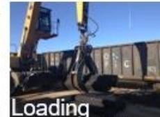
Post treatment inspection involves removing warped ties, making sure ties are not dripping, and ensuring careful handling during loading to prevent scarring or puncturing ties. Lab analysis investigates treatment penetration depth and retention via borings taken from treated ties. Borate diffusion is also verified (bottom right) via reagent spray appearing red in tie cut sections .
