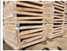
During drying, borates are diffusing into the interior of each wood tie as they migrate to remaining moisture. This creates a “reservoir” of borates that protects the ties from microbial degradation (i.e. fungi and insects).
