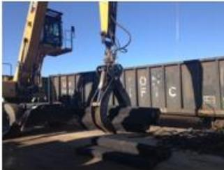
*Grappling ties in small bundles with the grapple ends extending below the bottom tie to "nest" the bundle is preferred*
